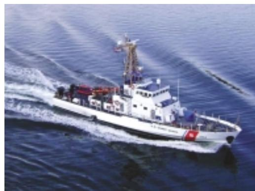
In corrosion testing conducted by the U.S. Navy, epoxy/polysiloxane coating systems, featuring products such as first-generation PSX 700 coatings, significantly outperformed 17 competing coating systems on topside naval systems. These applications are considered especially rigorous because of their exposure to high temperatures, seawater spray and exhaust gases.
